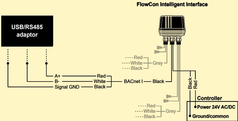
❶ Connect the 3 wires from the USB/RS485 adaptor to the black BACnet I cable of the FlowCon Intelligent Interface (middle gland).
